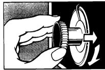
A. Push in the Control Knob and turn it to the right. It must be pushed in and turned only to the right (clockwise).
