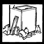
DO NOT let dust, lint, paper, rags, chemicals, etc., pile up around or under the appliance. DO NOT install the appliance against drapes or curtains.
